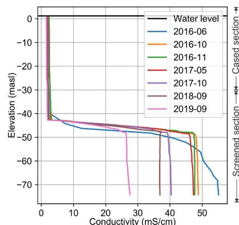
Figure 1. Electrical conductivity profiles from a monitoring well in the Magdalen Islands (F-2). Installation year : 2015.
