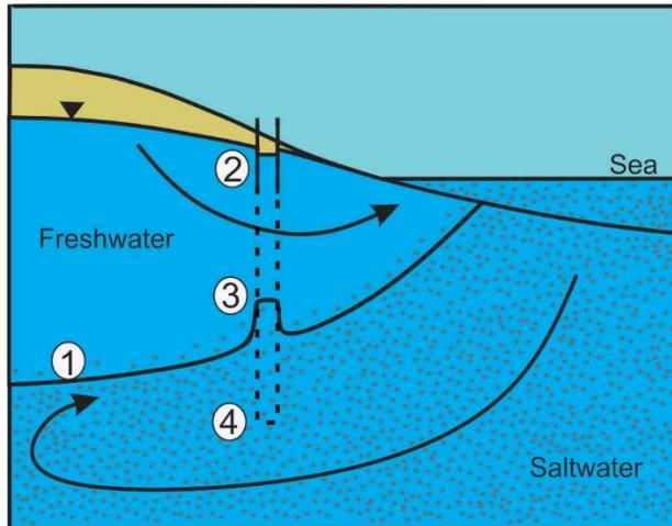
Figure 2. Conceptual model of groundwater flow in a coastal area highlighting 1) the freshwater-saltwater interface, 2) a drop of the water level inside the well, 3) the rise of the interface inside the well and 4) a decrease in the concentration of the saltwater inside the well.
