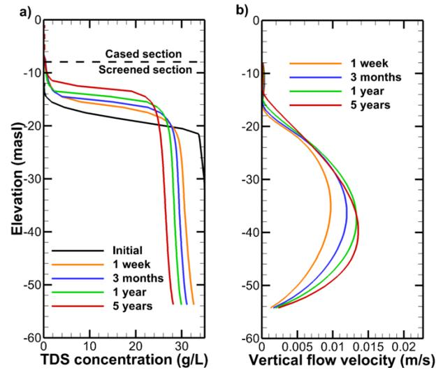
Figure 5. a) TDS concentration profiles over time (Scenario 1) compared to the initial profile without a well and b) comparison of vertical flow velocity profiles over time. A positive velocity indicates upward flow.
