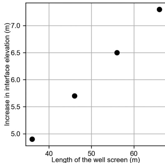
Figure 8. Change in the elevation of the interface for different well screen lengths after 5 years (Scenario 1, 8 to 10). (Elevation increase is with respect to the initial steady-state interface elevation without a well).
