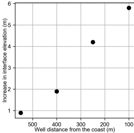
Figure 6. Change in the interface elevation within monitoring wells at different distances from the coast after 5 years (Scenario 1 to 4). (Elevation increase is with respect to the initial steady-state interface elevation without a well).
