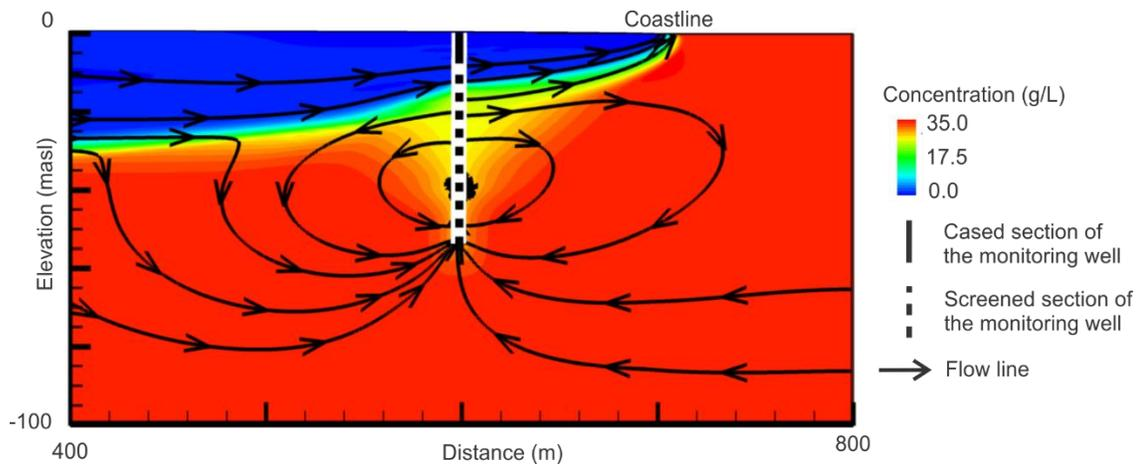
Figure 9. Cross-section of the 3D steady-state flow and transport simulation with an open monitoring well (Scenario 1). Note that the flowlines are based on the 2D (x-z) components of the 3D velocity fields but are nevertheless representative of the true flow patterns within the section. (Vertical exaggeration : 2x)
