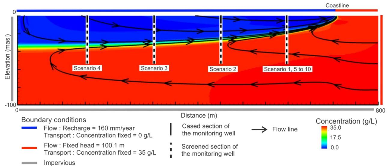
Figure 4. Cross-section of the steady-state simulation without wells, showing boundary conditions and flow lines. (Vertical exaggeration : 2x)
