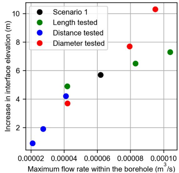
Figure 10. Simulation results of the increase of the interface elevation for different maximum vertical flow rates within the well (Scenario 1 to 10).
