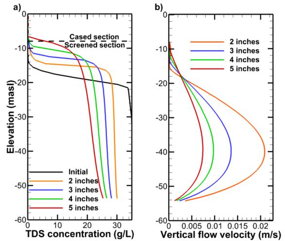
Figure 7. a) Comparison of TDS concentration profiles and b) comparison of vertical flow velocity profiles within different diameter wells, after 5 years (Scenario 1, 5 to 7)
